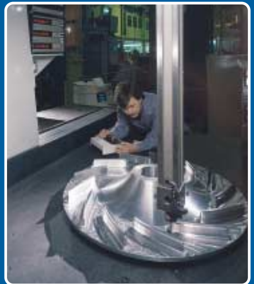
3-axis coordinate inspection system applied to a high-speed fan impeller
