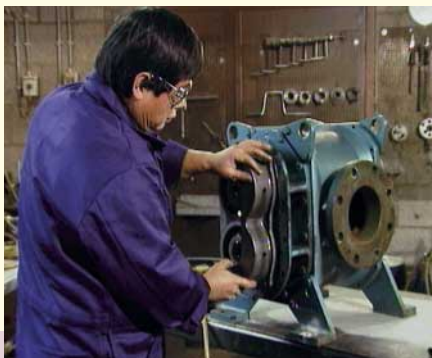
▲ Blower repair work.
