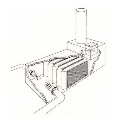
This approach removes completely the problems of noise break out and also reduces flanking losses considerably. Also, as the supply lines are also below ground there is no noise radiation form these.
