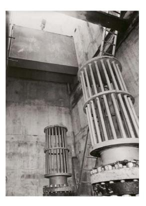
The above photograph shows a silencer under construction designed to vent 620,000 Nm3/hr of natural gas to atmosphere from 76 bar.
